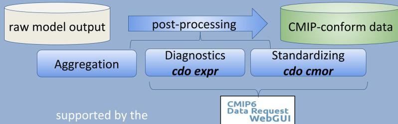
A highly modular infrastructure allows the user to customize the post-processing. The GUI supplies the user with tools to easily configure and automate the generation of parts of the post-processing. The post-processing interface requires specific raw model output file names.
