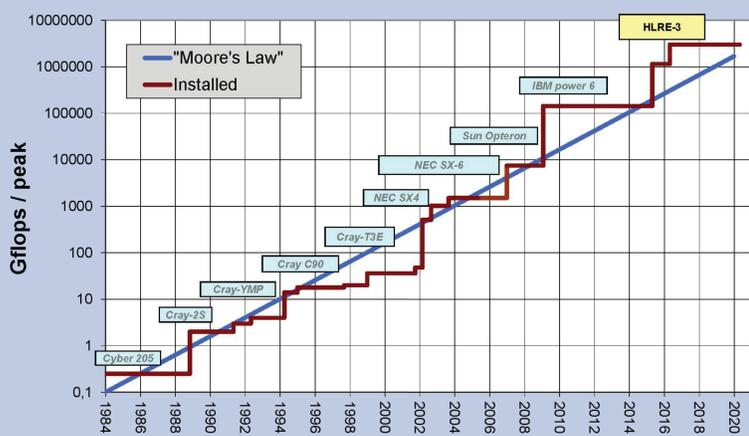
Since its foundation the peak performance of the supercomputers at DKRZ (red line, given in Gigaflops) has increase rapidly. It follows the projected rise of Moore's Law. (Graphic: DKRZ)
