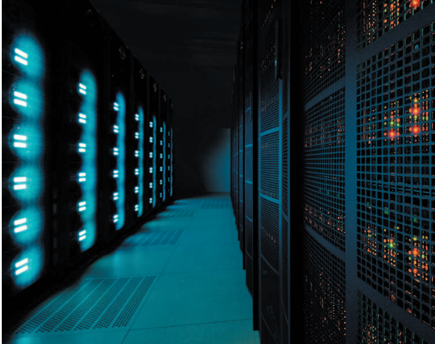
With the second stage of expansion in 2016, Mistral consists of ten such rows of computer racks – part of the hard-drive system (left) and the computational nodes (right) can be seen in the image above.
