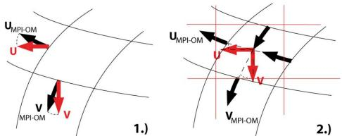
Rotation can be done by the cdo commands *rotuvb* and *mrotuvb* (the latter is not yet documented). *mrotuvb* combines the horizontal interpolation to the scalar grid with the rotation in one operator.
